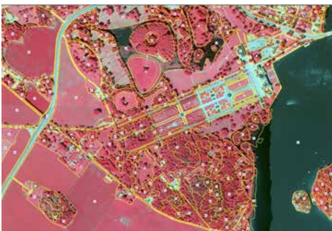
Colour infrared images provide the baseline for the biotope mapping of Stockholm.
