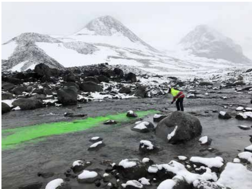
Measuring discharge in Tarfalajokk (using fluorescent tracer). Photo: Nimis Rosquist.
