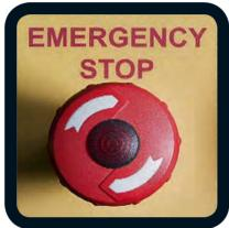
I would like to suggest that the feed tables be designed with better located E-stop buttons mounted on the inside of the side frames on both the operator side and the drive side of the feed table. Existing feed tables could be retrofitted with new controls.
