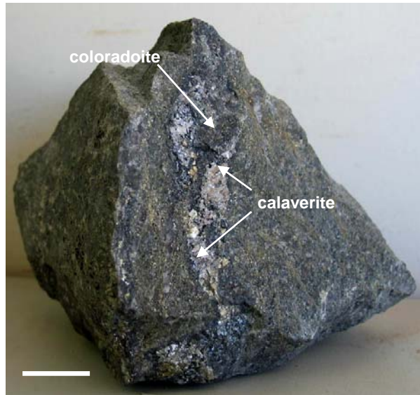
Fig 3. Stores 360 Bench. Hand specimen of Telluride. Scale Bar is approx 2 cm
