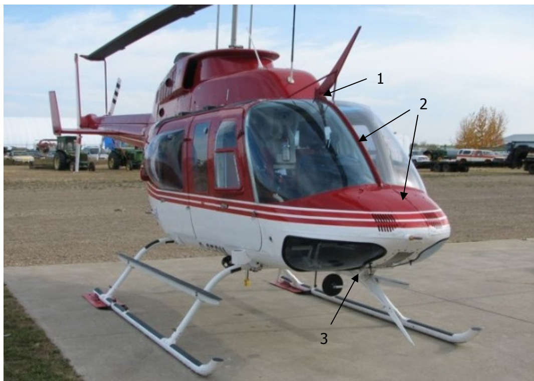
Figure 10: Bell 206 with WSPS. Upper cutter (1), windshield deflector (2), lower cutter (3).
