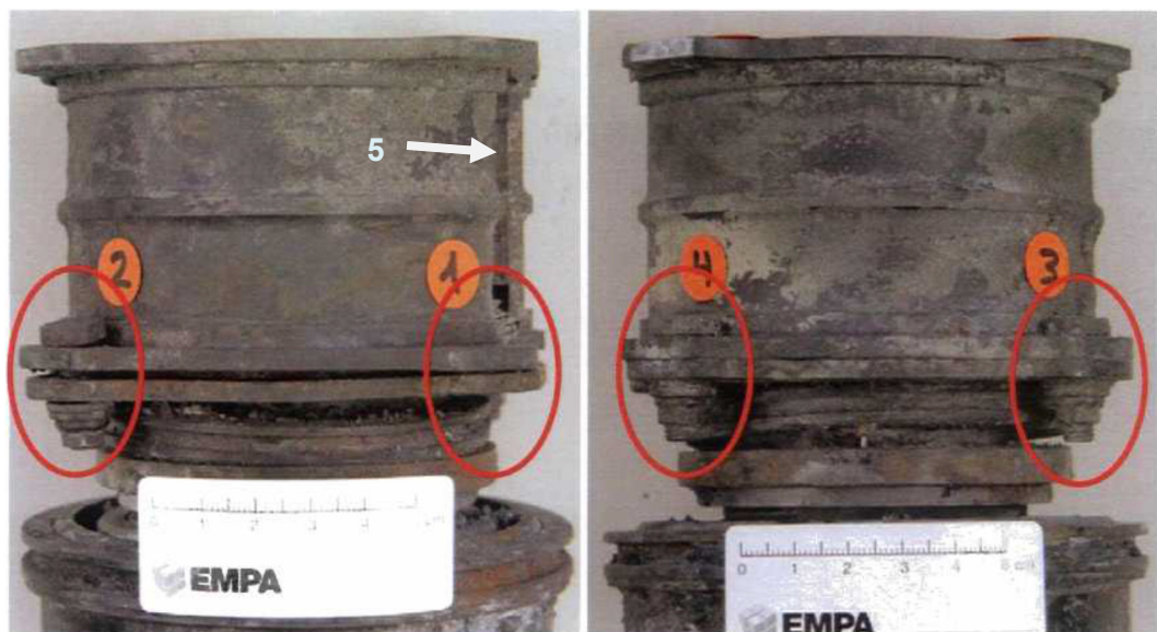
Figure 8: Missing bolt (1), loose bolt connection (2), intact bolt connections (3 & 4), missing tooth segment (5).
