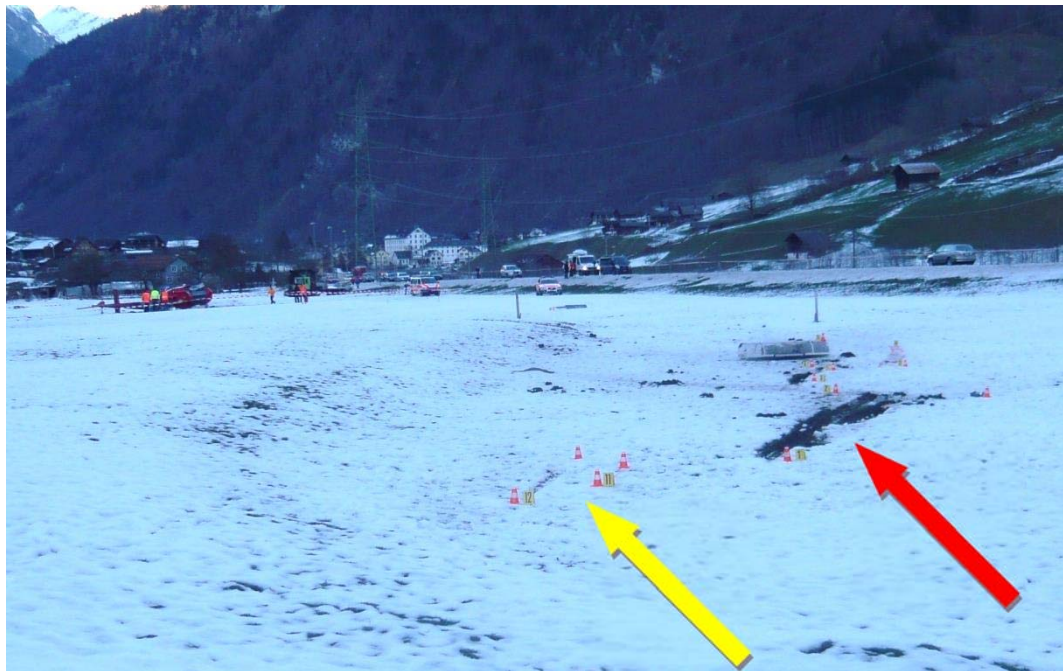
Figure 3: The first traces of impact from the right skid on the ground (red arrow) and traces of the tail skid and blade tips of the tail rotor (yellow arrow). Final position of the cargo basket and final position of the helicopter (photo from the day of the accident).
