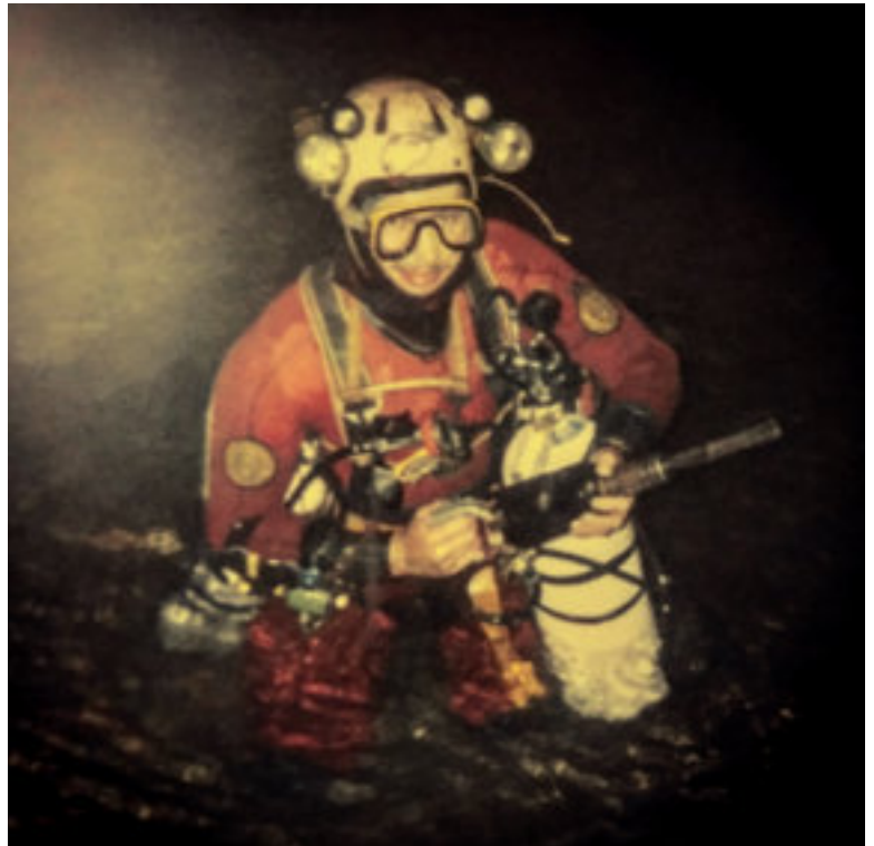
Robin Brown with CP9 air chisel. The large white cylinder is its air supply. (©Michael Thomas)
