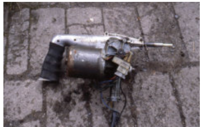
A Rawlplug Mechanical Hammer of the type I experimented with in the early 80s. And the modified version, complete with windscreen-wiper motor!
