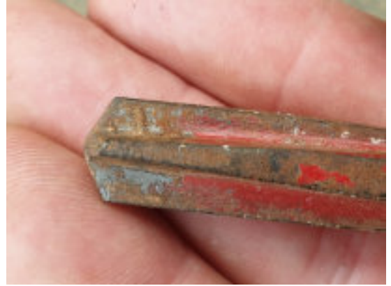
A rather knackered 1/2" star drill of the type we used to drill experimental holes by hand
