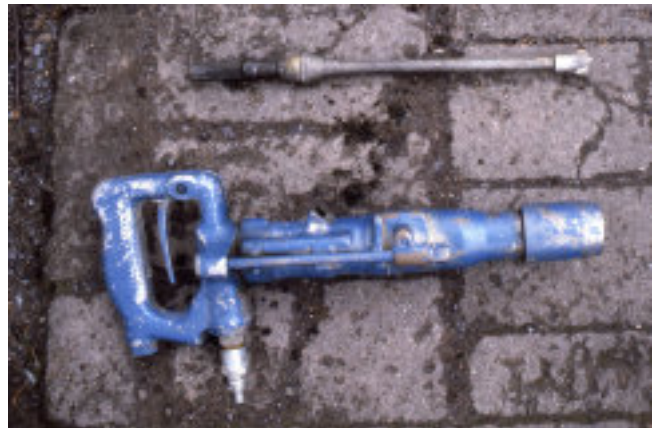
A small, compressed air drill similar to the one we planned to use with a diving cylinder.
