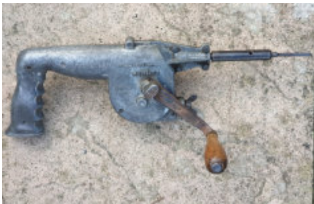
A Rawlplug Mechanical Hammer of the type I experimented with in the early 80s. And the modified version, complete with windscreen-wiper motor!
