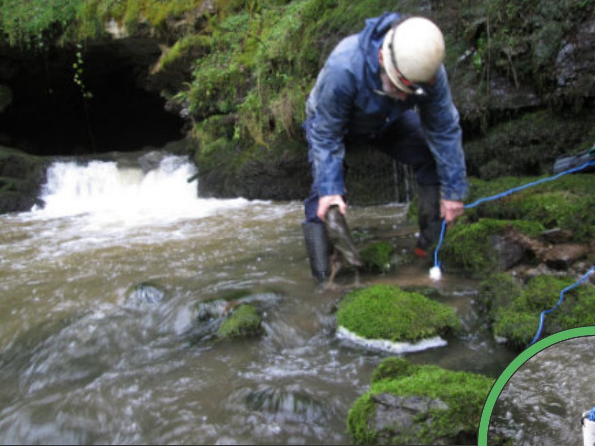
Jem Rowland placing a charcoal detector at the Dan-yr-Ogof resurgence (©Martin Hoff)
