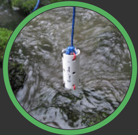
Charcoal detector, in protective sleeve, going into the river at the Dan-yr-Ogof resurgence (©Martin Hoff)
