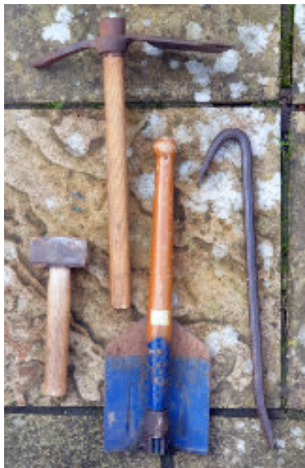
A selection of typical personal tools for digging. (©Bob Hall)
