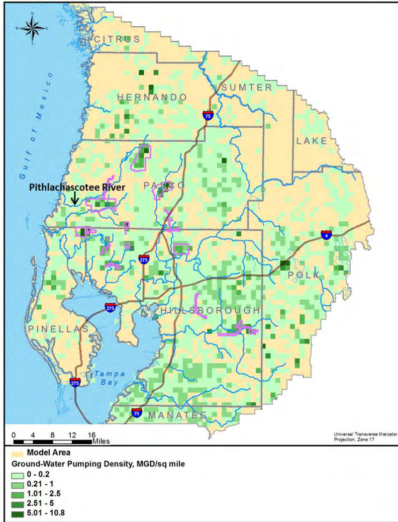
Figure 2-5. Average groundwater withdrawal rates in the geographic domain of the Northern Tampa Bay Integrated Model for the years 1989-2006. Boundaries of wellfields operated by Tampa Bay Water shown in purple. Image modified from Geurink and Basso (2013).
