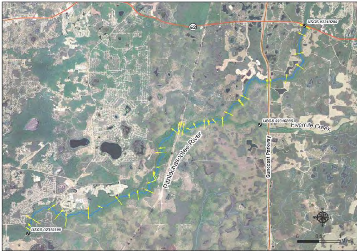
Figure 4-5. Location of the HEC-RAS cross-sections and U.S. Geological Survey gages in the freshwater reach of the Pithlachascotee River (image reproduced from Engineering & Applied Science, Inc., 2010).
