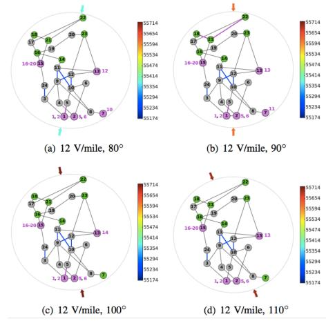
Switched off lines are colored magenta and the IDs of unused generators are labeled beside their connected substations
