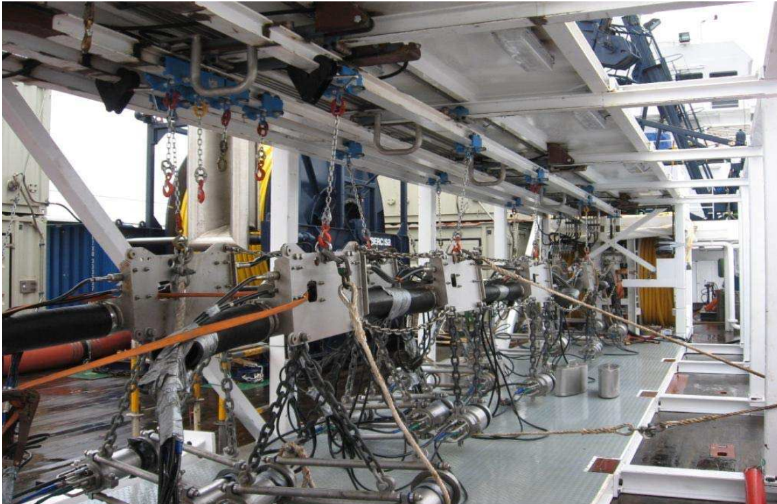
Fig. 2. 10 - Airgun working frame designed and mounted by the “Marine Technology Unit” of CSIC (Spain) for the RV Sarmiento de Gamboa. The airgun array consists of 6 Sercel GGUN-II canyons distributed in three clusters of various capacities, hanging from a float (Vázquez et al., 2012).
