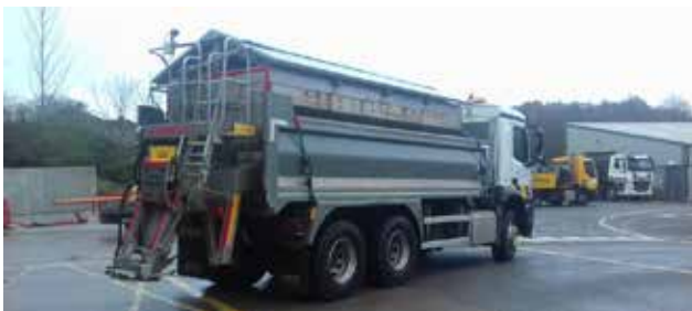
9 cubic Metre salt spreader mounted on 26 tonne Tipper Truck
