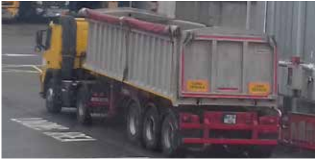
30 Tonne aluminium trailer unit for drawing road salt from the ports to the Council salt barns
