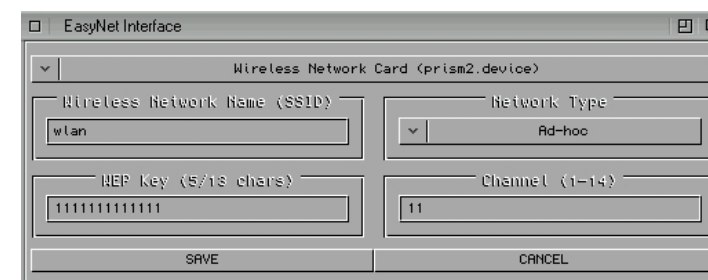
Setting up your wireless card to access an WEP encrypted network is easy thanks to Amigakit's EasyNet interface.
