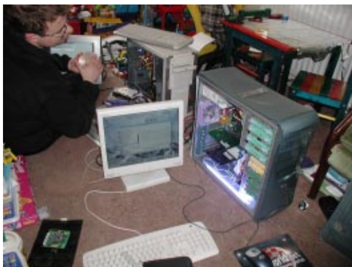
It's alive!! Sven of Stellar Dreams tests Mick's AmigaOne after the new CPU module has been fitted.
