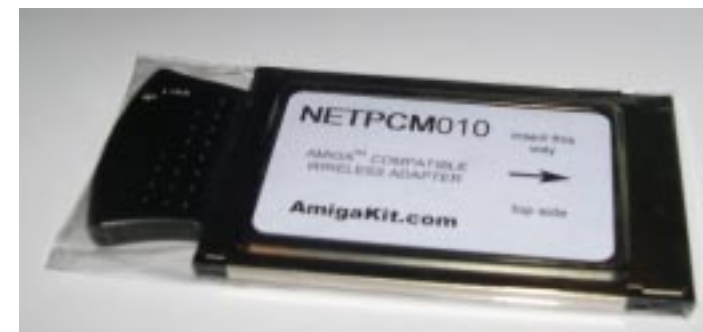
The NETPCM010 wireless card is compatible with the A1200 and A600 and works with standard 802.11 wireless networks.
