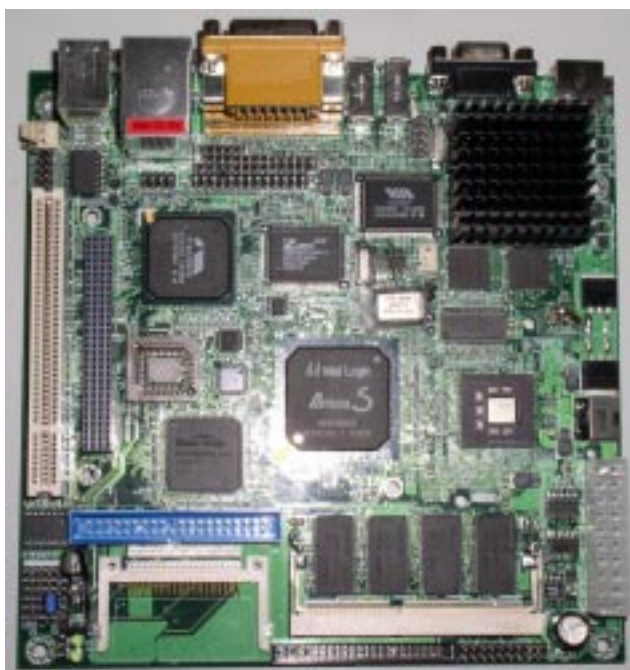
A pre-production µA1-I. Notice the Compact Flash slot (bottom left) and the soldered on CPU (middle right).
