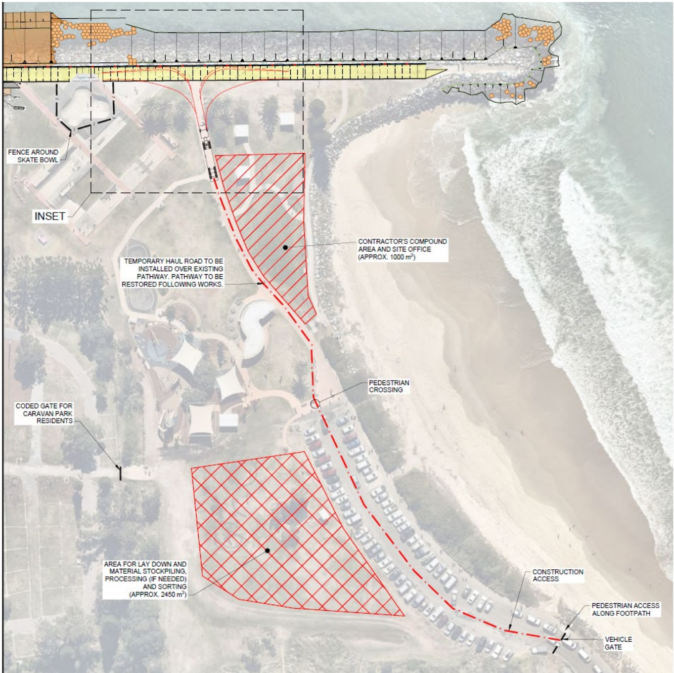
Figure 8: Proposed on-site stockpile site and temporary construction compound located near proposed project footprint (Source: Royal Haskoning DHV, March 2022)
