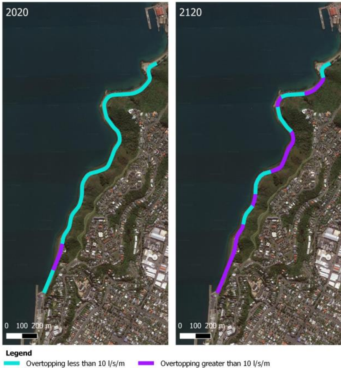
Figure 6-2: High level overtopping summary along the project site for present day (left) and 2120 (RCP8.5) (right) sea levels during a 1%AEP storm event
