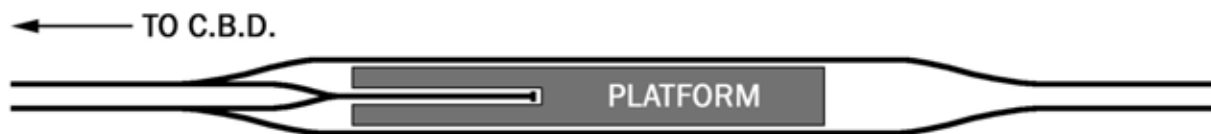
Figure 4.3.1: Bay platform for short-turning trains
