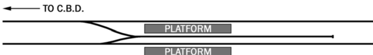
Figure 4.3.2: Intermediate terminal with split platforms
