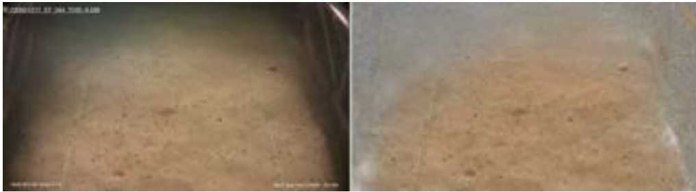
Figure 4: Original frame (left) and time-averaged HSL correction (right). Spotlight effect evident in the original image in the upper left of the image. Spotlight not longer evident in processed image, only the seabed remains in focus for analysis.
