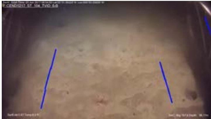
Figure 9: Laser detection. Screenshot of the laser detection algorithm in one of the frames. Long and mostly vertical edges are detected as blue lines. The two longest lines correspond to the position of the lasers and further extrapolation with a line fitting allows to define a polygon in the central region. Notice that sometimes the sledge was visible at the edges of the video, which resulted in the identification of false positives.
