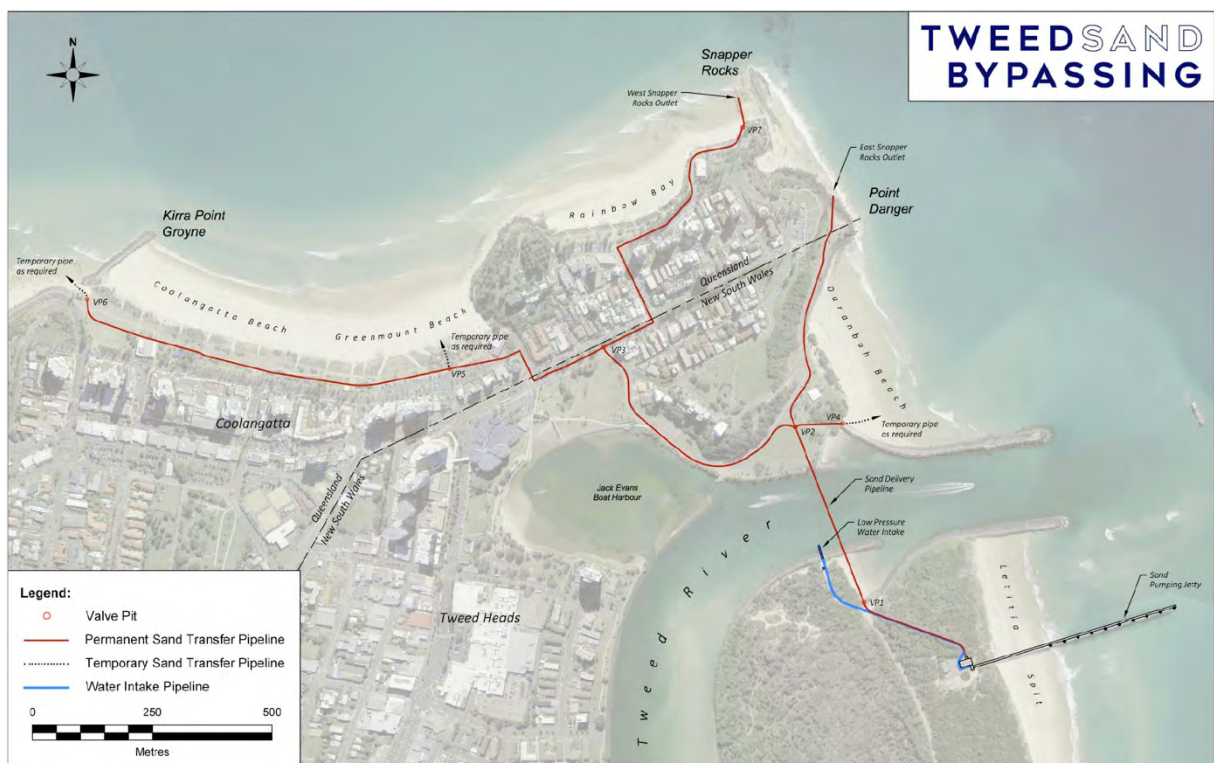
Figure 1.1 Fixed sand bypassing system (TSB, 2020)
