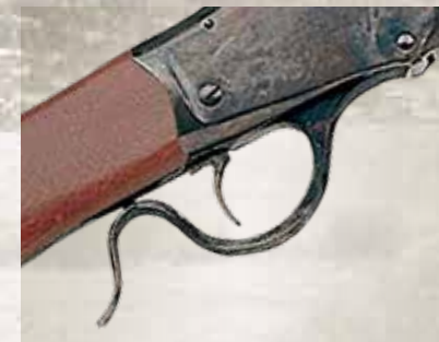
The 1885 High-Wall's loading lever (left), opens or locks the rifle's falling-block action (right).
