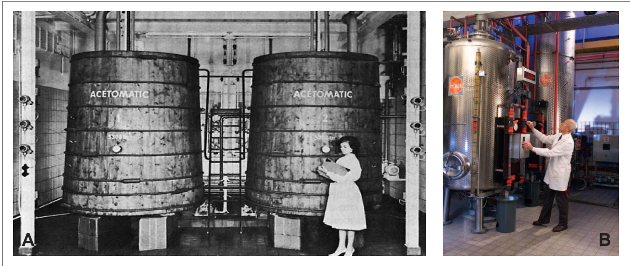
Fig. 10: Submerged acetification systems.
