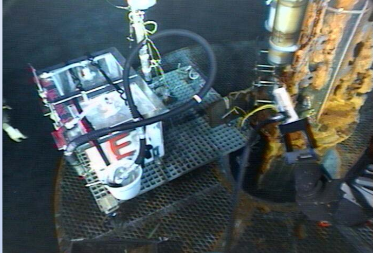
Basement fluid collection
