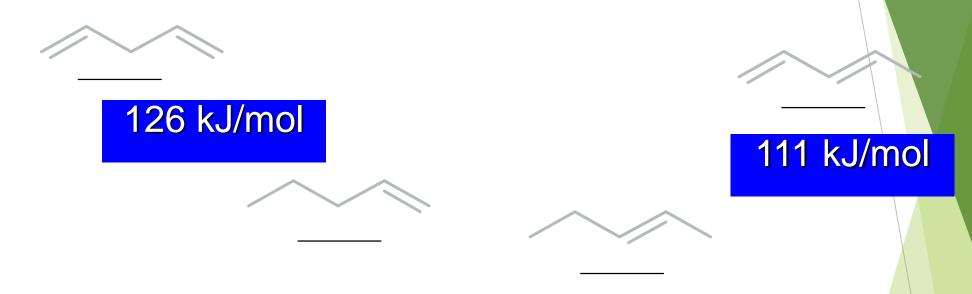
when terminal double bond is conjugated with other double bond, its heat of hydrogenation is 15 kJ/mol less than when isolated
