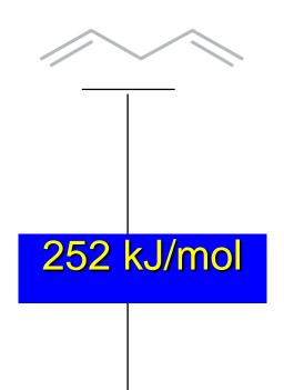
▶1,3-pentadiene is 26 kJ/mol more stable than 1,4-pentadiene, but some of this stabilization is because it also contains a more highly substituted double bond
