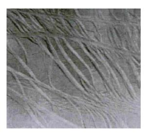
Relation of stretcher strain in stress-strain curve
