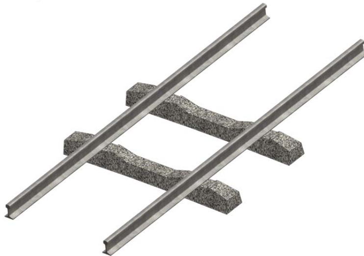
Fig. 5. The assembly of cross-ties with rails
