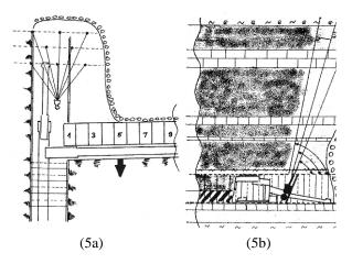
**Fig. 5**. Crossing of the longwall and the transportation drift (5a) and the vertical section of coal seams and the blastholes along the drift (5b)
