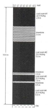
Fig. 4. Vertical section of the coal seams.
