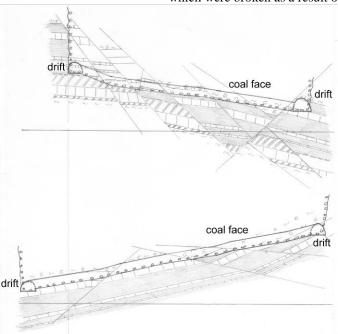
**Fig. 1**. Longitudinal sections of two longwalls, cutting mostly country rocks due to their momentary unfortunate position.
