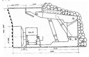
**Fig. 3.** Cross section of a longwall equipped with sublevel caving shields type VHP742/1 and ESA-60L shearer
