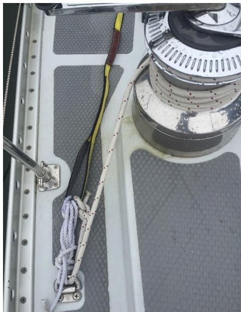
Figure 6-4 Tensioning the Jacklines
