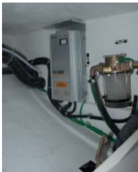
Figure 4-9 Battery Charger, Seawater Strainer, and Engine Seawater Intake Seacock; port locker aft of engine box
