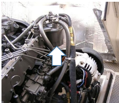
Figure 4-4 Secondary Fuel Filter (top center)
