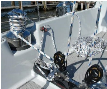
Figure 1-10 Mainsheet System; Traveler, Winch and Cleat
