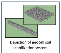
deployed directly in water at the shoreline and disseminated broadly across combat forces. The SUBMAT utilizes a geocell soil stabilization system with soil nail anchors.
