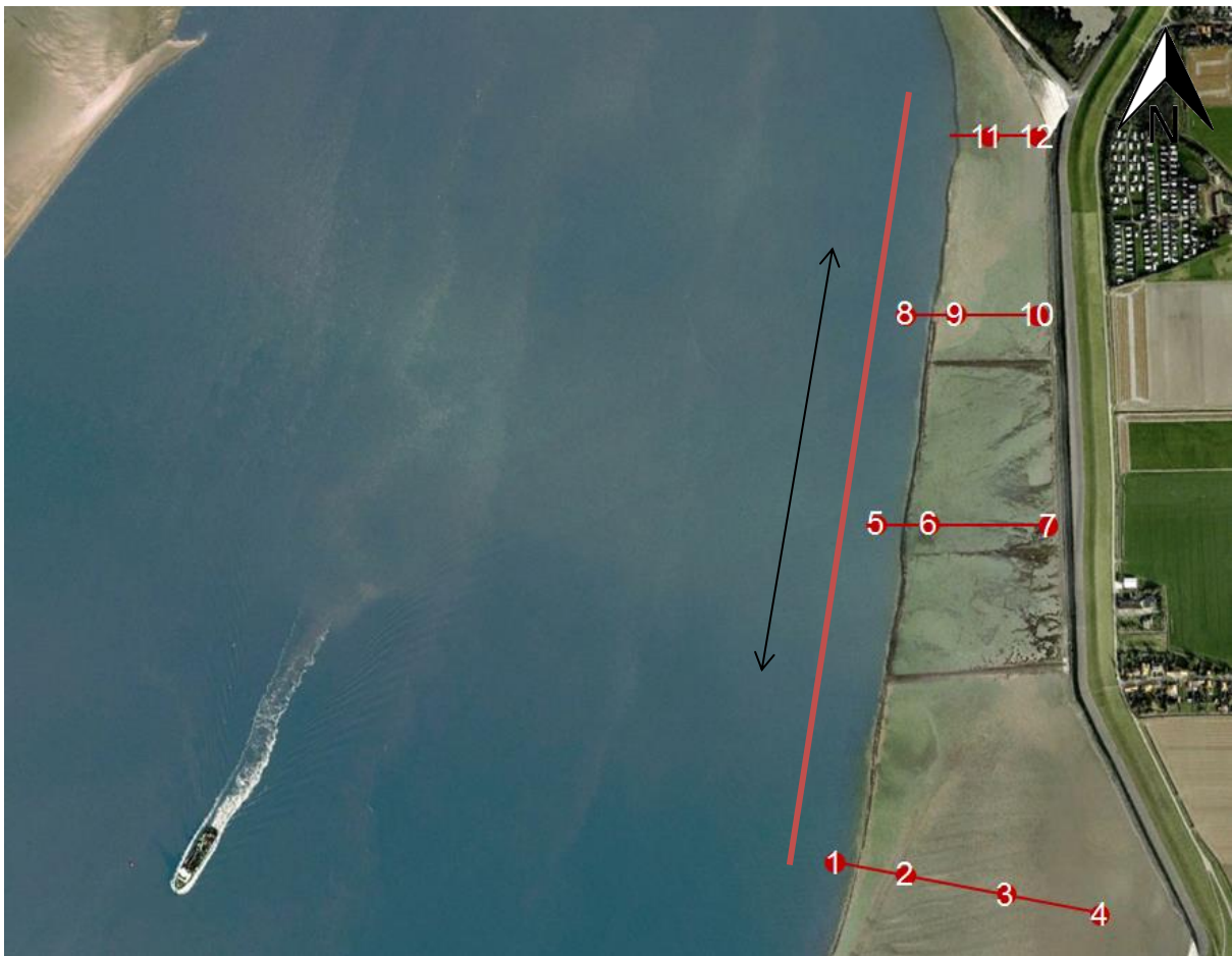
Figure 3.3 - Flow measurement points at Knuitershoek. The flow measurement transect is shown by a red line.
