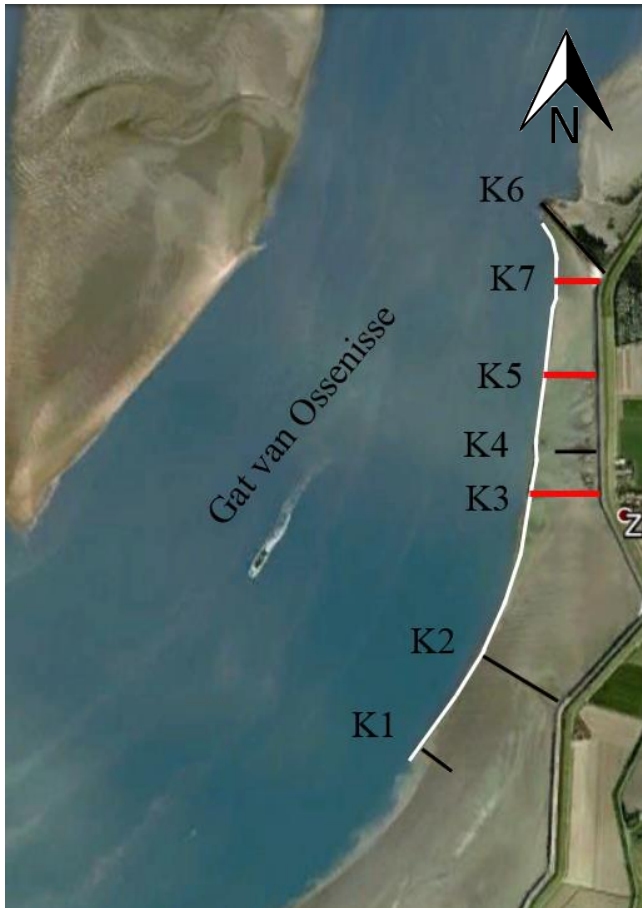
Figure 2.7 - The design at 'Knuitershoek'. The red lines represent the heightened groynes (K3 & K5) and the new groyne (K7) (Background picture: Provincie Zeeland, 2016).
