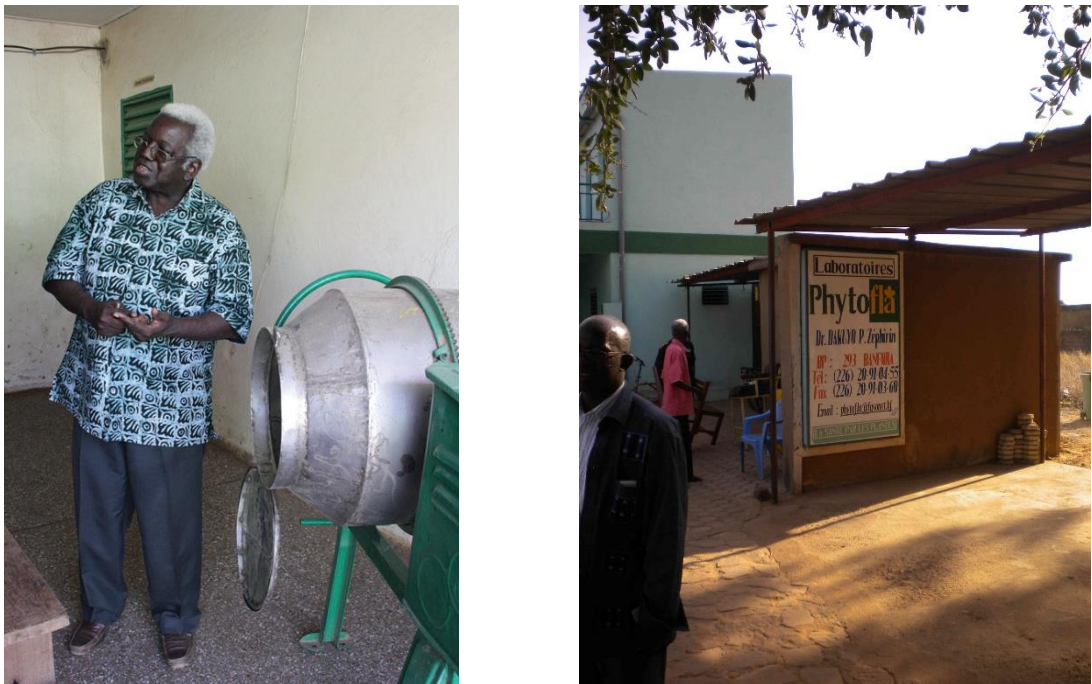
Figure 4: Dr. Zéphirin Dakuyo demonstrating a self-constructed machine for producing homogenous mixtures of medicinal plants (DAKUYO et al., 2015) and the outside of the Phyto Fla laboratory.
