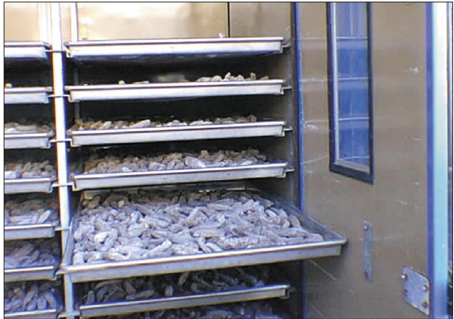
Figure 7. Oven used for the final drying of sea cucumbers.
