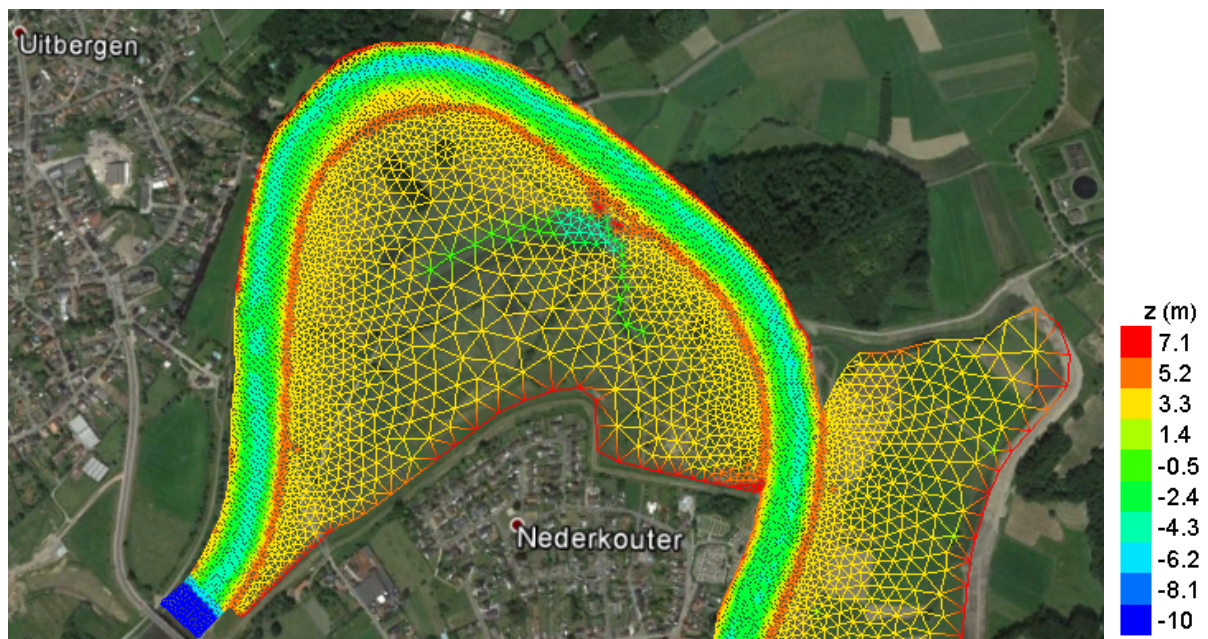
Figure 7 Planview of part of the computational domain to model the FCA-CRT in Bergenmeersen. The colour scale represents the bottom elevation values (m).
