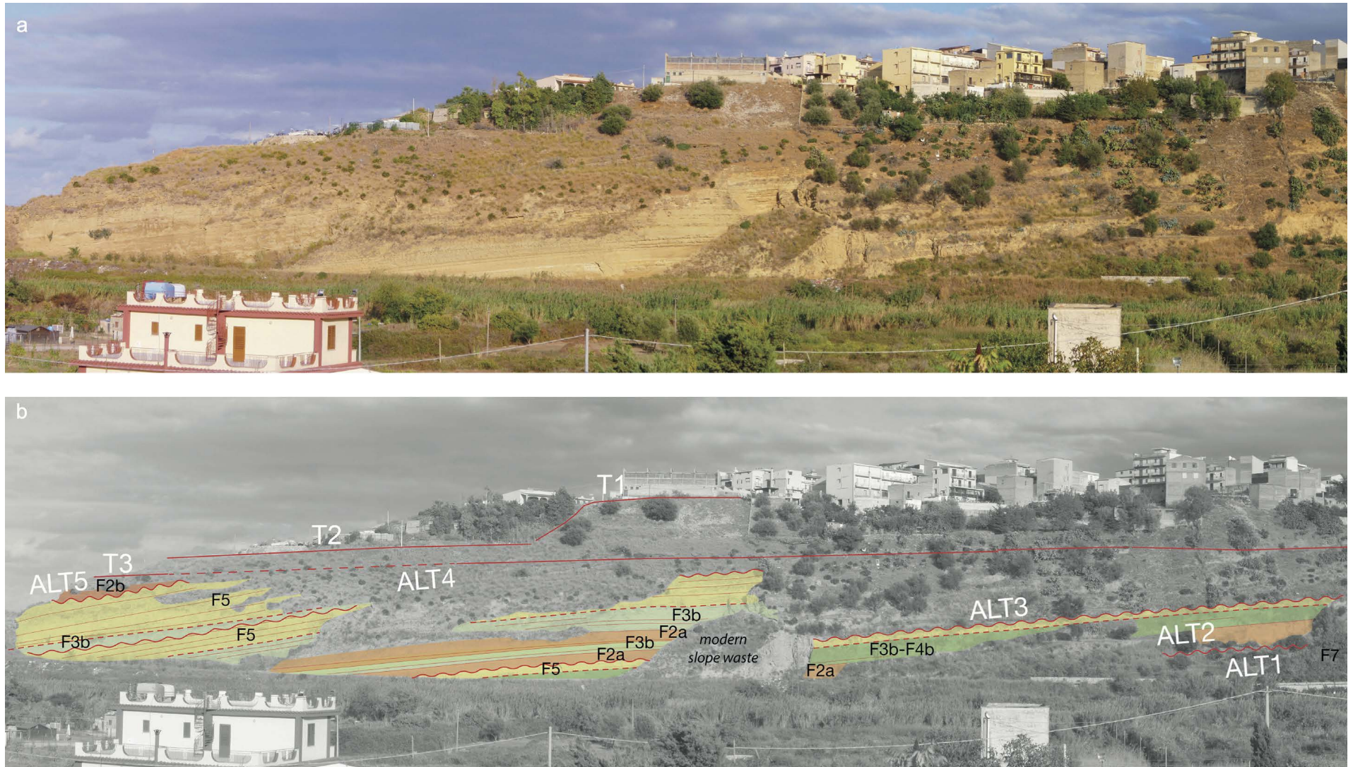
Fig. 6 - (color online) Stratigraphic cross section of the Altavilla unit at Altavilla (See Fig. 1 for location). a) Panoramic view of the section. b) Interpretation of sedimentary patterns, showing onlap and downlap geometries (thin red lines), sequence boundaries (ondulating lines) and surfaces of maximum flooding of individual EDSs (dashed lines); the Altavilla composite section (uppermost 65 m of the log in Fig. 2) was based on five logs measured and described along this outcrop.
