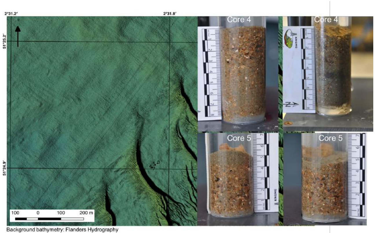
Figure 37. Shallow cores (4 and 5) and seabed samples (7 and 8) taken by divers in the barchan dune refugium area. RV Belgica campaign ST1919. Core 4 predominantly had shell hash in the top 2.5 cm. Finer-grained material is mixed in, as well as silt-clay layers and organic material (right). Core 5 has a coarse seabed matrix as well, though clearly shows deposition of fine-grained material at the top.
