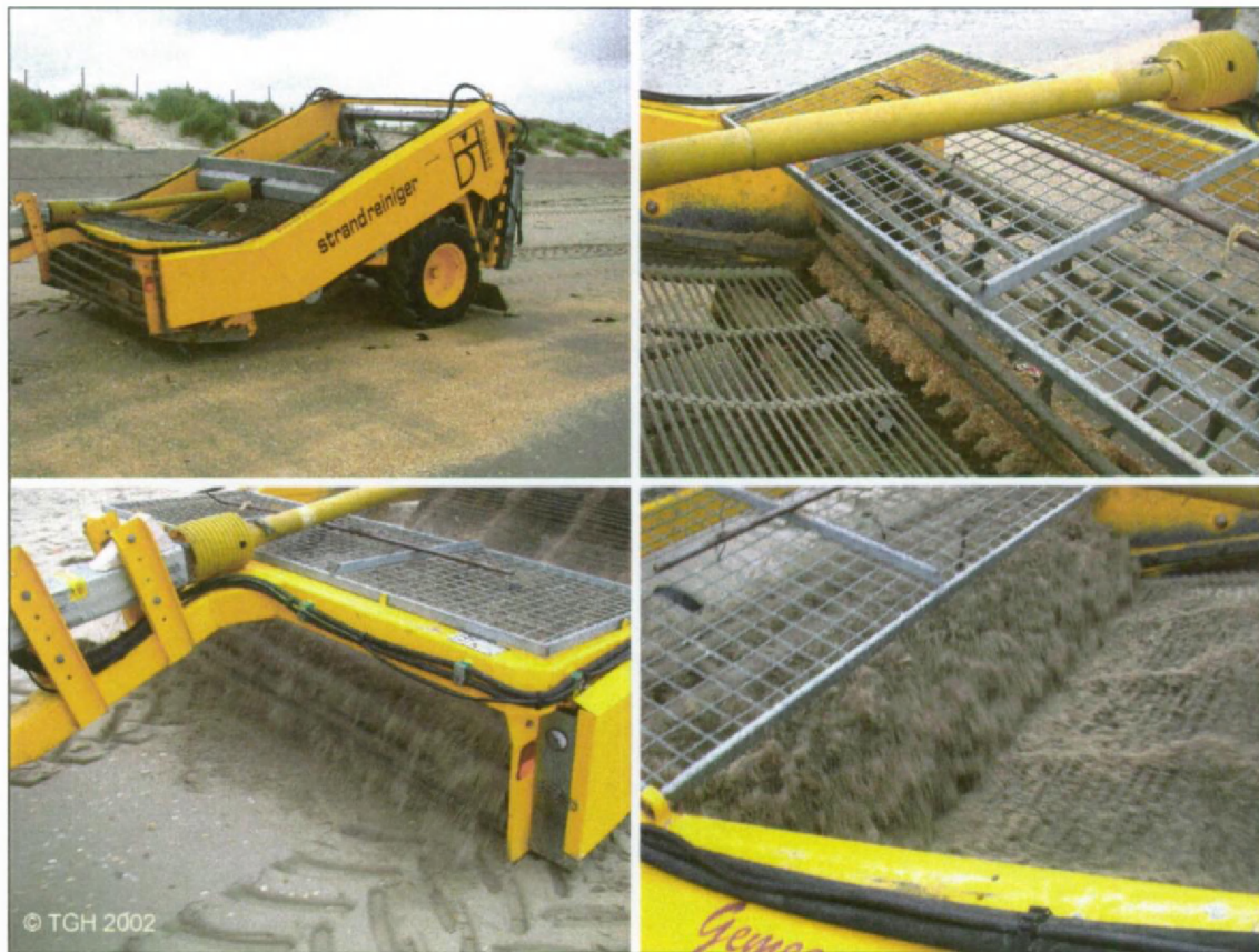
Photo 1: One of the most used types of mechanical beach-cleaners; the Hurricane-Eco type ® .
