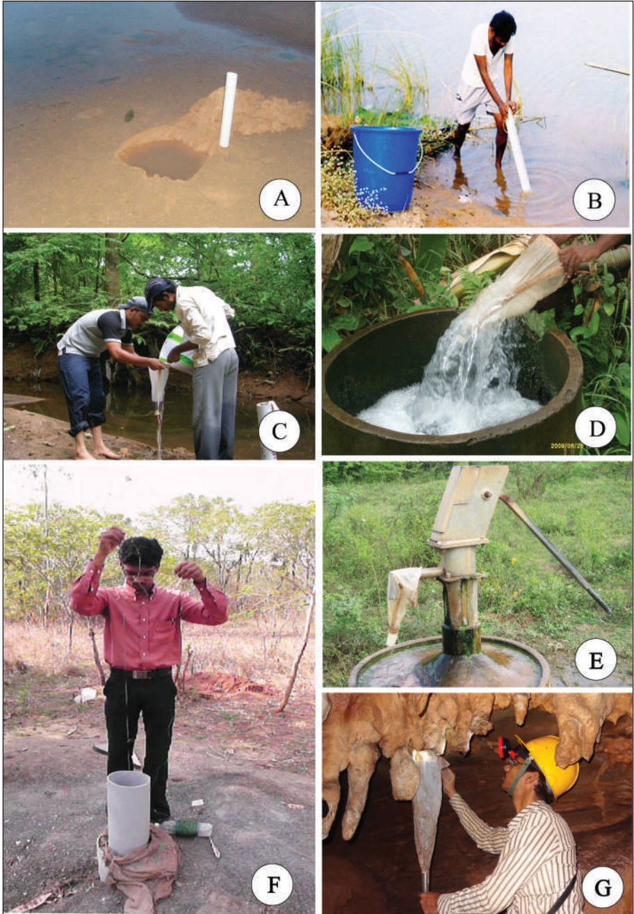
Fig. 1. Different types of sampling methods. (A) River bank, Karman-Chappuis method; (B) R. Godavari, direct coring method; (C) Filtering supernatant of core sample; (D) Direct filtration of water pumped out of an agricultural borewell; (E) Water from a hand-operated suction pump filtered through plankton net; (F) Sampling a newly dug-out borehole; and (G) Direct filtration of drippings from cave ceilings (here, stalactites).
