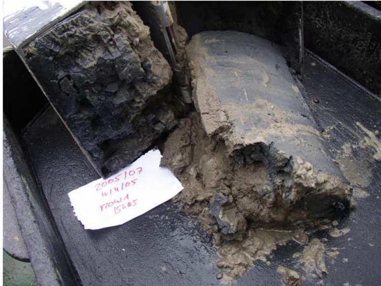
Figure 2.1: Van Veen grab sample of Holocene layered clay covered by a thin layer (5 cm) of fine sand with patches of recent ('liquid') mud, west of Pas van het Zand, R/V Belgica campaign 2005/07.
