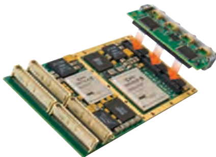
AXM modules attach to PMC Modules with user-configurable FPGAs.
