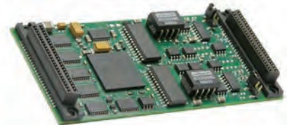
Acromag offers more than 40 IP modules to perform analog I/O, digital I/O, serial communication, CAN bus, Mil-Std-1553, and configurable FPGA functions.
