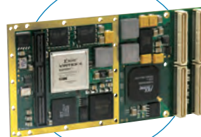
The base board is ready for conduction-cooled applications.
