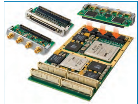
AXM extension I/O modules plug into a mezzanine connector on many Acromag FPGA boards to provide additional I/O signal processing capabilities.
