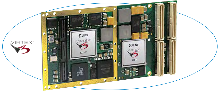
Download your own programs into the reconfigurable FPGA to quickly create custom I/O module. Optional I/O modules plug into the front mezzanine.
