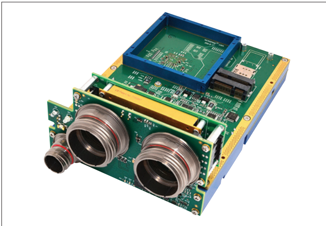
ACEX-FP-01 front panel with ACEX-FP-PF power filter/bridge board mounted on an ACEX-4610 single-width carrier card
