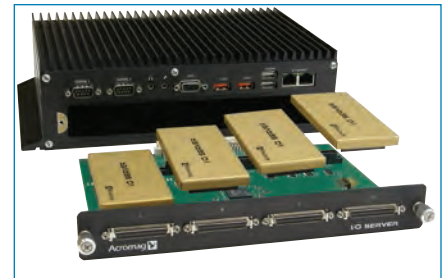
IOS modules plug into an I/O Server's integrated carrier
