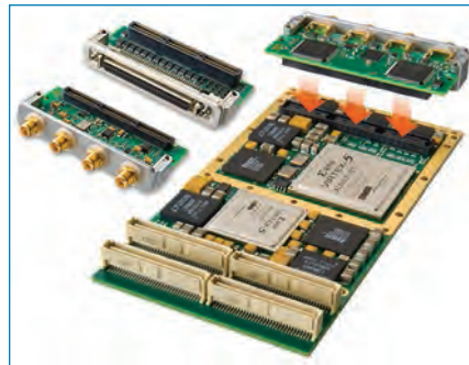
Plug in an AXM analog or digital I/O module for additional I/O signal processing capabilities.
