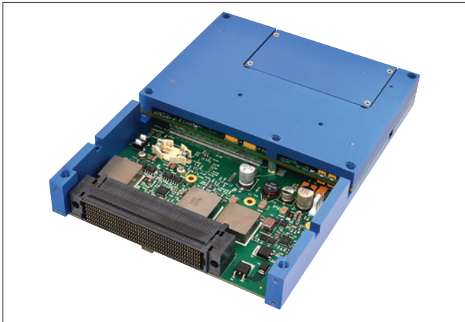
ACEX-4610 single-width carrier card shown with optional ACEX-CC-01 conduction cooling kit rails and XCOM-6400 COM Express module
