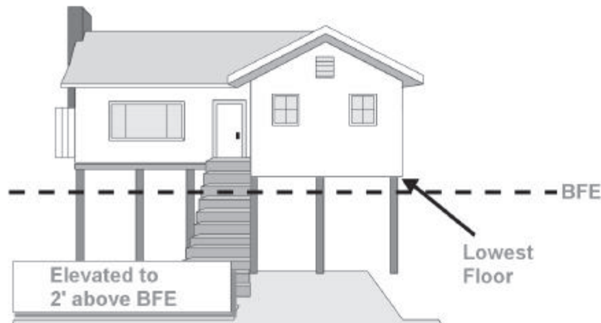
Figure 7-12. Repaired—elevated 2 feet above BFE; actuarial rate: $216
