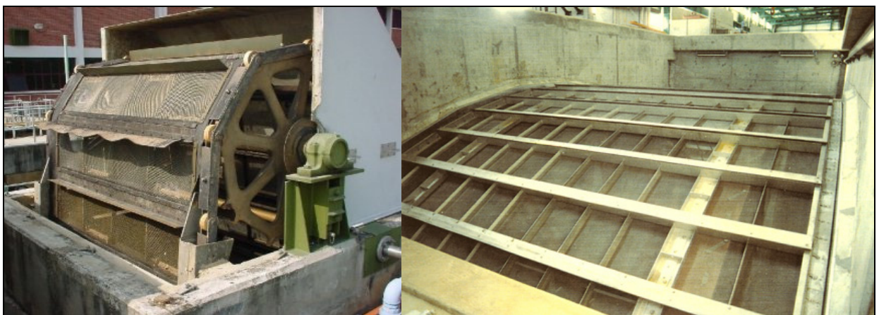
Figure 6-18 Examples of travelling band and drum screens 5
