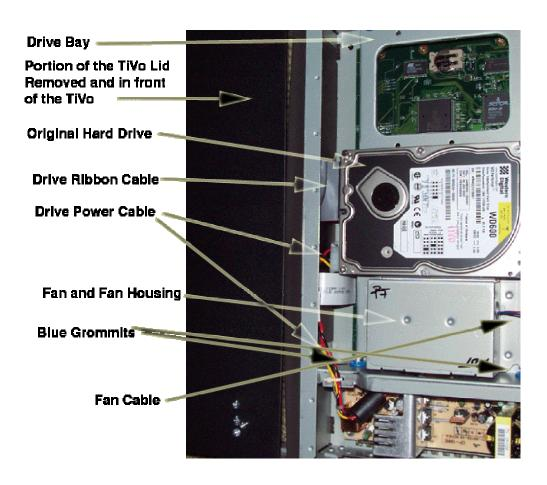
(a) The hard drive has a power connector running into the hard drive. The power cable has a white connector plugged into the hard drive. Remove the power
