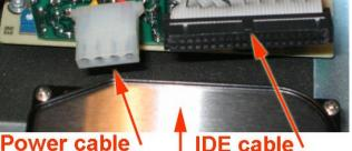
Power cable \ IDE cable \ (flat side down) (notch on top) Top of hard drive
