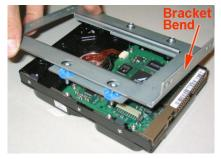
Put the new drive and bracket back into your TiVo by aligning the holes in the bracket with the posts in the TiVo and sliding the bracket forward. Then screw in the two screws that you removed from the TiVo bracket back into the bracket with your Torx T-10 screwdriver.
