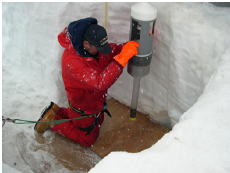
Figure 17. The Alfred-Wegener-Institut gravity corer deployed at HWD Sites 1 and 2. The hole through the ice sheet is covered by plywood in this image.
