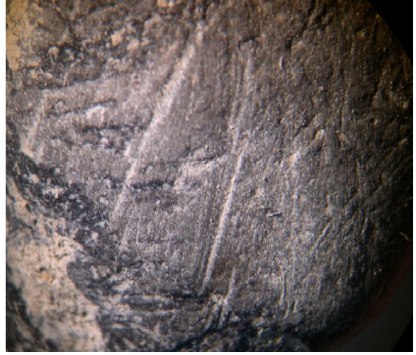
Figure 22. Features in the core from Site 1: Striae on pebble 20 mm across found at 35-37 cm bsf
