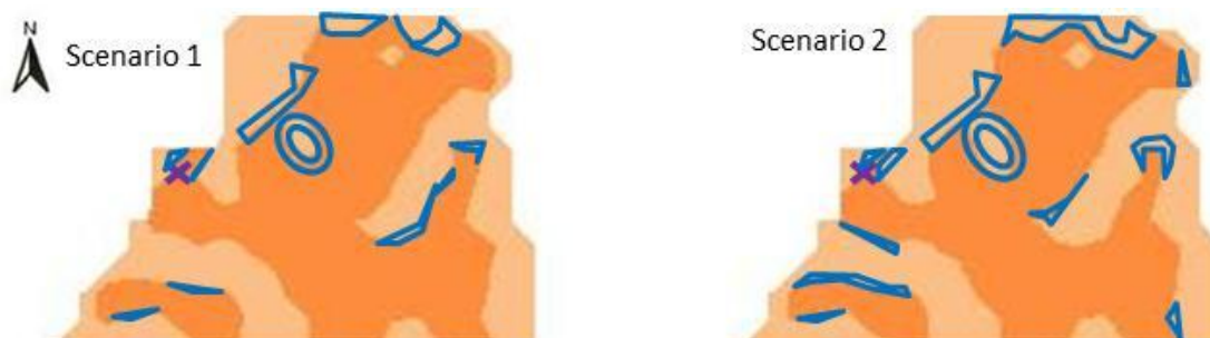
Figure 2.26 Projected 2040 rainfall “risk” maps for the Castries study area based on the algorithm used in the landslide hazard map. The areas denoted by blue are projected to experience a decrease in hazard. The purple “x” approximately marks the downtown Castries, Source: we produced these maps based on data from McSweeney et al., 2010; Hijmans, 2005.
