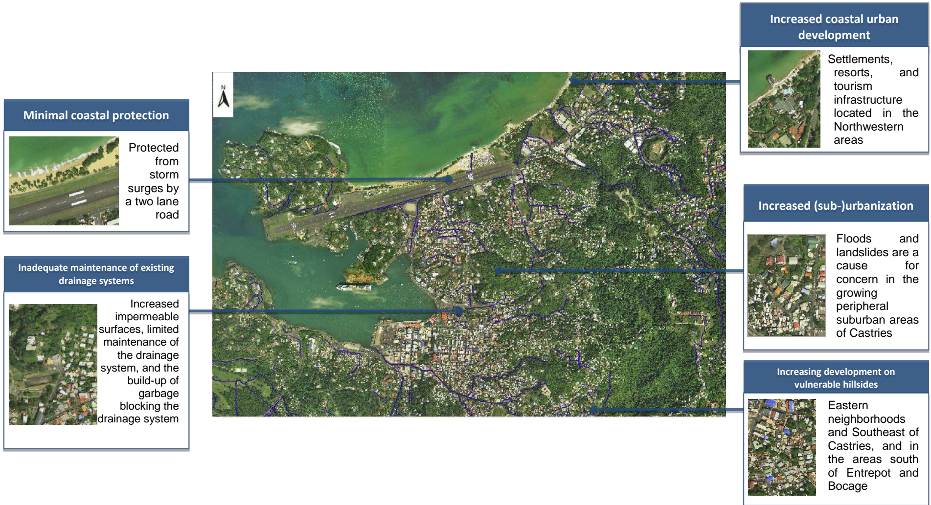
Figure 5.1 Predominant features of the built environment in Castries that impact upon flood and landslide hazard risks.
