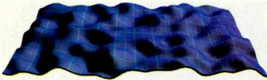
FIG 2— QUASI-RANDOM VIBRATIONS OF NXT DISTRIBUTED-MODE SPEAKER DIAPHRAGM.
