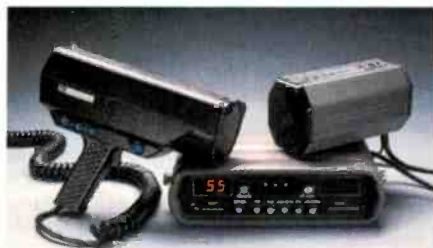
The Kustom Signals HR-8 and KR-11, two of the many radar units that can be operated in an instant-on, or “pulse” mode.
