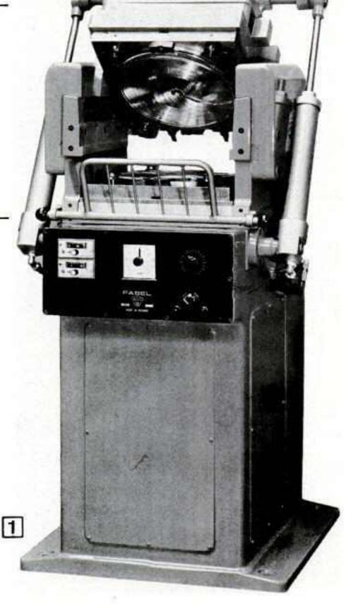
■ with the new automatic Super FABEL TC ■ the only record press with all transistorized thermocontrol system and ■ the recent modern automatic extruder mounted in compact unit with the press.
