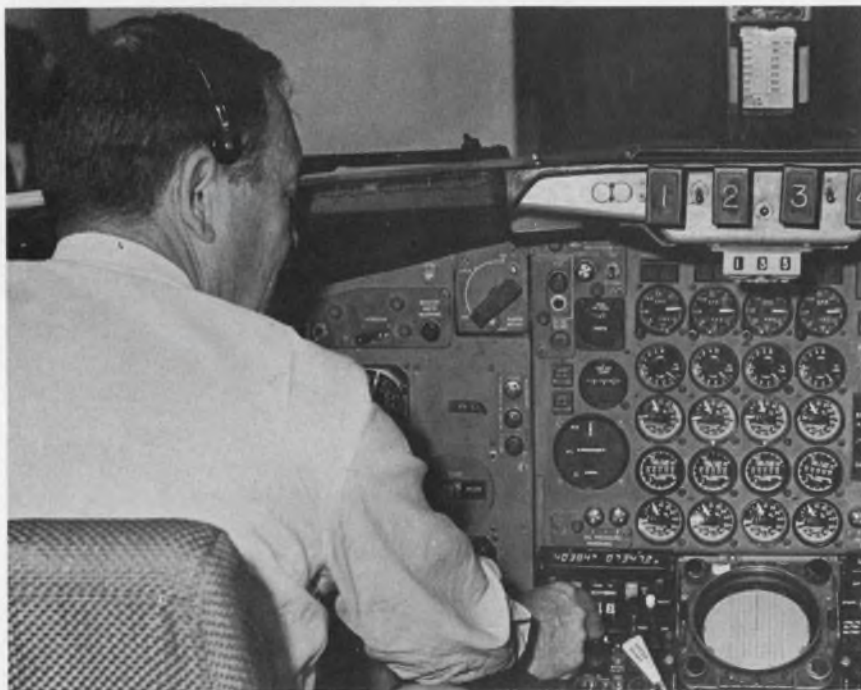
Inertial navigation equipment is adjusted before take-off by Pan American World Airways pilot, Capt. D.L. Combs. The Sperry SGN-10 system, which is being installed on the first of 70 Pan Am airliners, is completing engineering evaluation tests. The airline hopes to receive Federal certification for the equipment this year.
