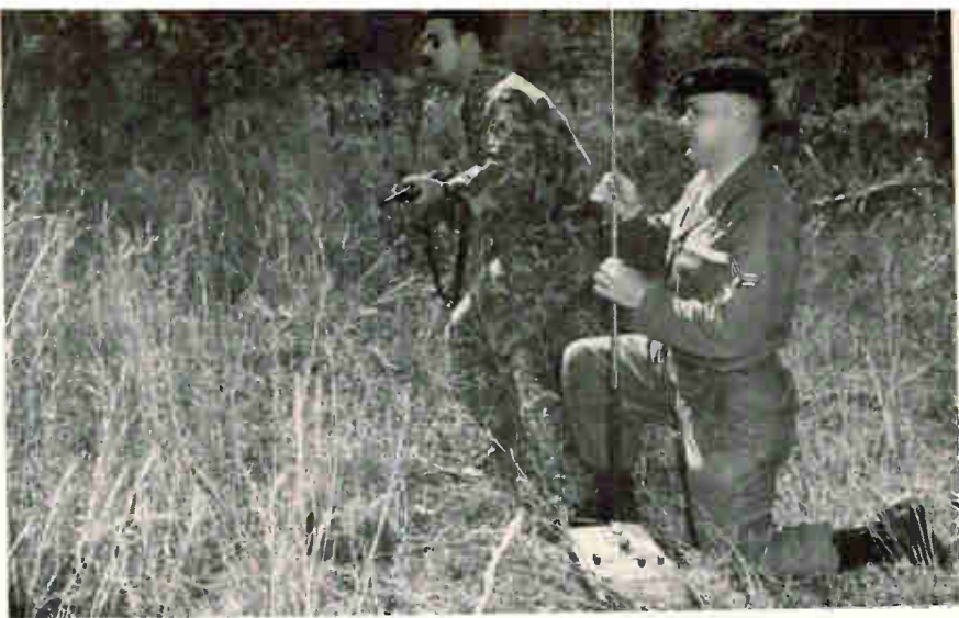
Homing beacon HRT-2, used to mark drop- or landing-zones, is portable and operates at low frequencies. The Special Air Warfare Center would like something cheaper.
