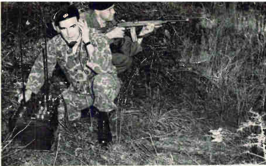
Forward air control radio pack, manufactured by Sylvania Electronic Systems combines four transceivers and is light-weight, but has at least one drawback—it's expensive
