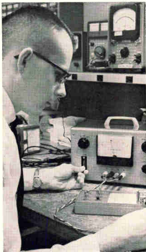
Typical test setup for measuring leakage current. Colored line shows extra bootstrap lead required for checking decoupled stage.
