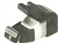
cartridge has a 15 degree vertical tracking angle, induced field moving magnetic armature, and is fully compatible for stereo or mono operation. Other information from their specifications include: Standard 47,000 ohm load impedance, 4 coil system to aid eliminating hum pickup, easily replaceable stylus assembly, low dynamic mass, high stylus compliance, low needle talk, and wide stereo channel separation.
