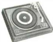
According to information supplied by Garrard, the SL72B is a synchronously powered automatic turntable highlighting a new low mass tubular aluminum hexagon shaped tonearm that floats virtually friction free on needle pivots within a gyroscopically gimballed mounting. The fully adjustable counter-weight is isolated from the arm to damp out resonances.
