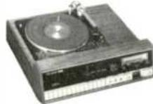
Slide controls for volume, balance, bass and treble. Volume range switch for improved low level listening. Direct-plug-in modular circuitry. Altec's Fail-Safe Electronic Protection System. Convenient push-button controls for power, FM, AM, phono, auxiliary cassette, high filter, mute, loudness, mono, volume range, speaker 1 and speaker 2. Front panel microphone inputs and tape recorder gain controls. Spring loaded terminals for main and remote
