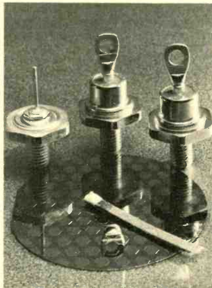
PROTOTYPE SCHOTTKY DIODES made by a new technique. These are 50-volt, 50-ampere units. In the foreground is a disc of the hexagonal silicon substrates used in the rectifiers. At left is a diode without its protective cap, showing how the metal to semiconductor contact is made.
