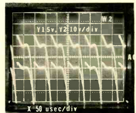
FIG. 5—GOOD WAVEFORMS of transformer pin 2 (upper trace) and the grid of the horizontal output tube (lower trace).
