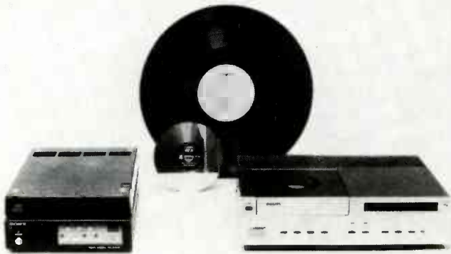
THE COMPACT DIGITAL DISC, as compared to a 12-inch L.P. Actual diameter of the disc is 4.7 inches (12 cm). Shown in the right foreground is the Philips player and in the left foreground is Sony's new player.
