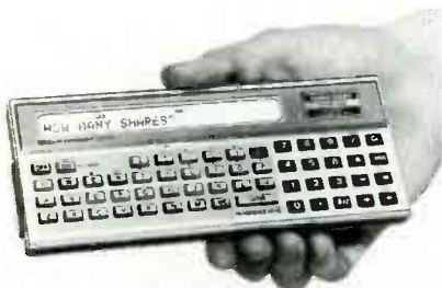
FIG. 1—LIQUID CRYSTAL DISPLAYS for alphanumeric use, such as the one in Radio Shack's TRS-80 Pocket Computer, are becoming commonplace. They are not suited, however, for graphics purposes.
