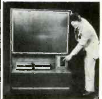
THE 50-INCH SYLVANIA SUPER-SCREEN television system uses a black matrix screen, which offers sharply improved contrast under bright lighting conditions.
