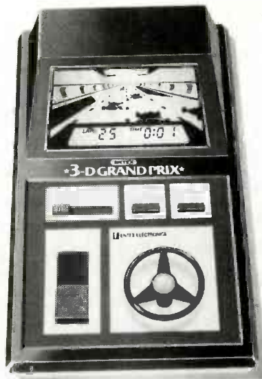
FIG. 2—LCD's CAN BE USED for graphics, as in Entex's 3-D Grand Prix game, but the displays are “hard wired” and cannot be changed by the user.
