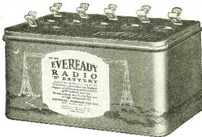
Eveready "B" Battery No. 766. 22½ volts. Six Fahnestock Spring Clip Terminals, giving variable voltage from 16½ to 22½ volts, in 1½-volt steps. Length, 6¾ ins.; width, 4¼ ins.; height, 3 3/16 ins. Weight, 5 lbs.
