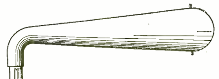
Fig. 8. General method of expanding the vibrating column of air as used in phonographs.
